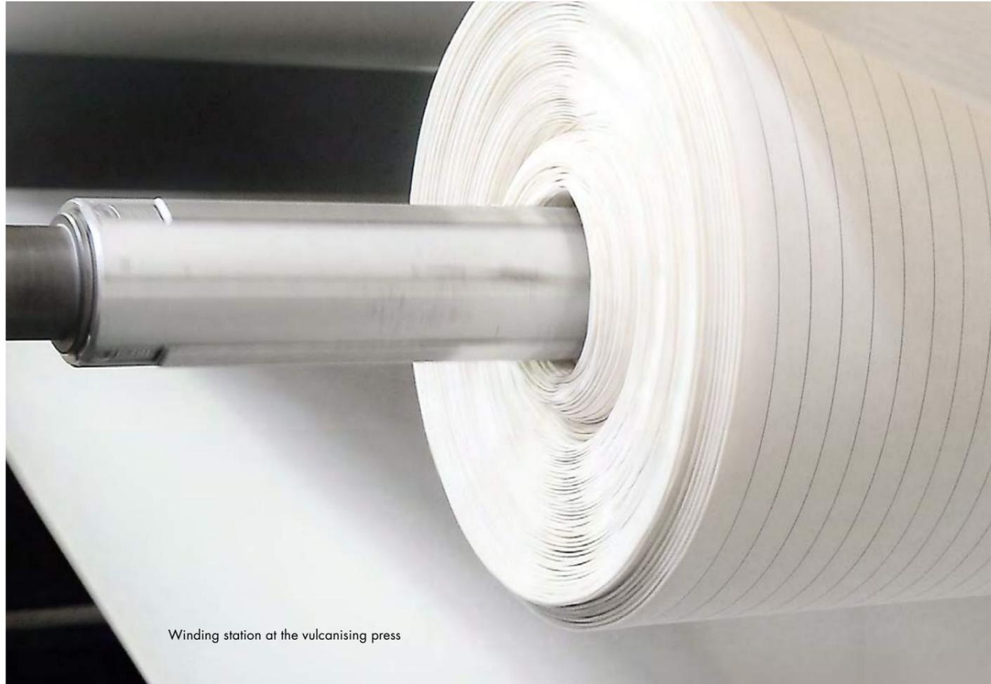
Winding station at the vulcanising press
