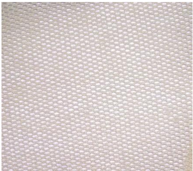
8330 Meta-Aramid Mesh Weight: 100-106g/m2 Width: 198-203cm
