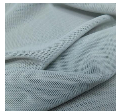
6580 Polyester Mesh Weight: 189-229g/m2 Width: MIN 92cm
