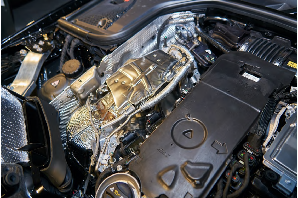
Figure 3: Heat protection with high heat-resistant adhesive bonding: Heares adhesive is particularly suitable for flexible bonding of aluminium and glass fibre fabric or for heat protection in the exhaust tract: glass fleece into shaped stainless-steel sheets. (Foto nolax)
