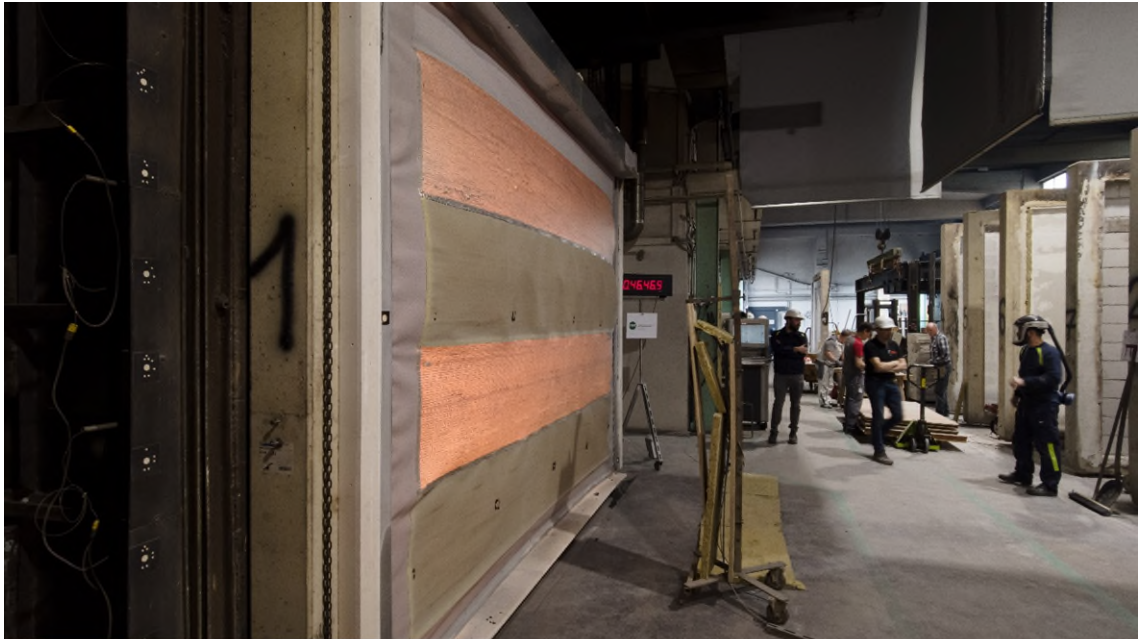
Figure 1: EW test (DIN EN 16034) carried out in March 2022 at IBS in Linz. The laminate coated with Heares (glass fiber fabric/Heares adhesive/aluminium foil) withstood the heat ( > 900\text{ }^{\circ}\text{C} ) for 60 minutes. (Photo nolax)
