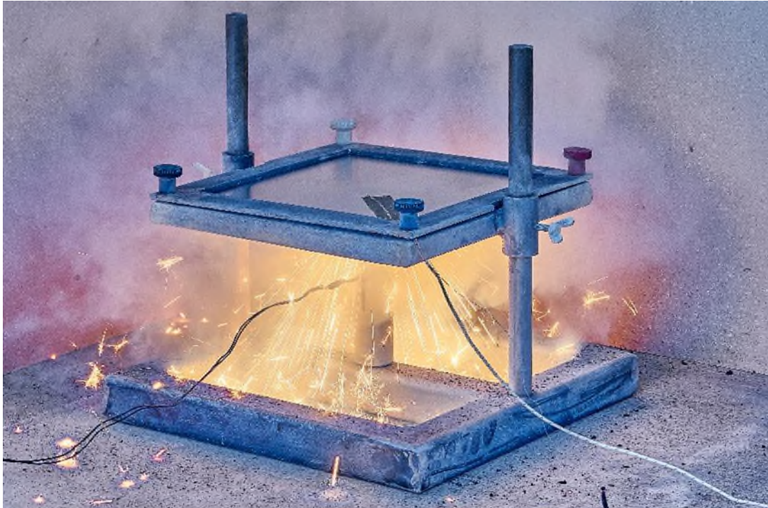
Figure 2: Impact by means of a fountain firework in nolax's own test rig (temperature: 1300 °C, duration: 20 s, distance between fireworks and test specimen: 30 mm). The result: No burnthrough of the test specimen after 20 seconds.
