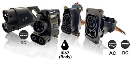
The Combined Charging System (CSS) is a standard for charging electric vehicles, which uses Combo 1 and Combo 2 AC/DC inlets which can be used with both AC and DC connectors to provide power at up to 200 Kilowatts. These inlets and connectors are an extenstion of the IEC Type1 and Type 2 inlets & connectors, with two additional direct current (DC) contacts to support high-power DC fast charging. CCS connectors support DC charging only.
