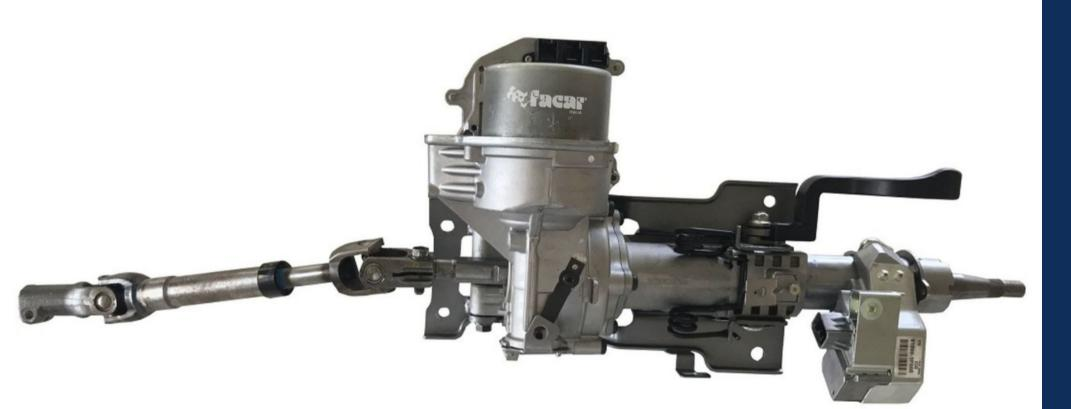
The electric steering column (EPS) has replaced the power steering system in small and medium sized cars and has become the most used solution on segment A, B, and C cars due to its efficiency, reliability and compact structure. Located directly behind the steering wheel, on the steering column, it consists of a control unit, an electric engine and a torque sensor, and provides assistance in wheel rotation, based on the speed of the car and the force applied to the steering wheel.
