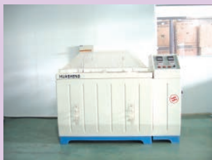
盐雾腐蚀试验箱 Corrosive salt spray chamber
