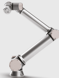
Cobot, kooperativer Roboter
