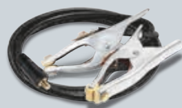
Double earth clamp 25 mm², 3 m, 350 A 070714
