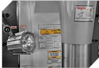
Moveable work lighting lamp
