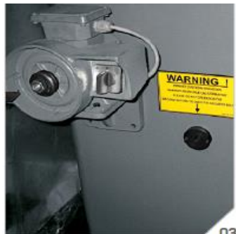
Çakı bileme motoru (ekstra ekipman) Diamond (tool) dresser (to sharpen the chip breaker) (extra equipment)
