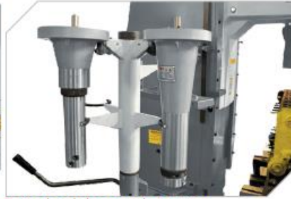
Boring head changer robot system
