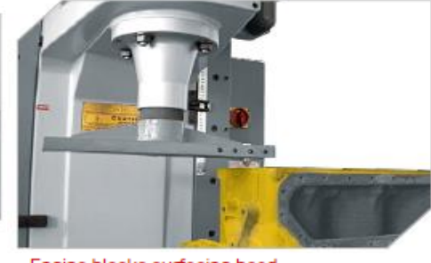
Engine blocks surfacing head
