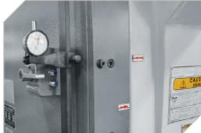
Depth dial gauge control apparatus(except dial-gauge) and limit switches
