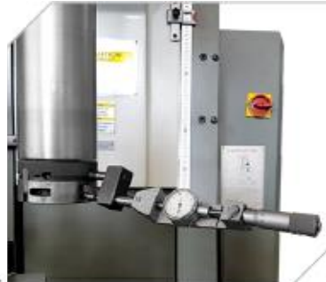
Paso mikrometresi (ekstra ekipman) Feed dial gauge micrometer (extra equipment)
