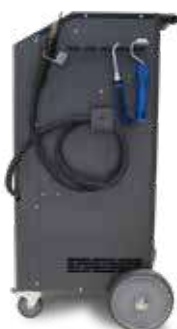
SIDE WITH ACCESSORIES SUPPORT AND AIR GUN
