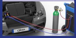
Kit for connection of 200 bar bottle to A/C Station - Inclusive of:
