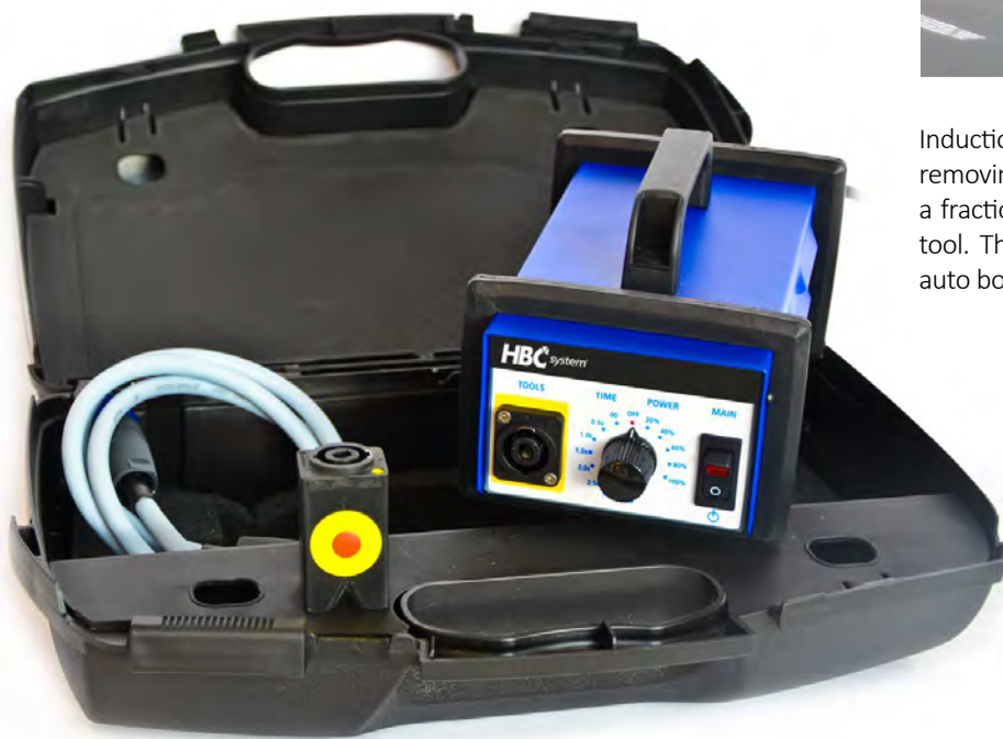
Part no. 17500 Electro-Magnetic Dent Removal System
