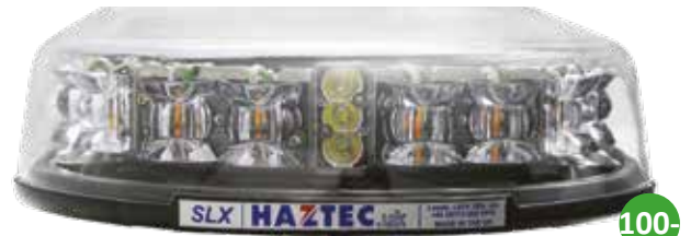
XEX four module end unit with optional 100-10423 alley light
