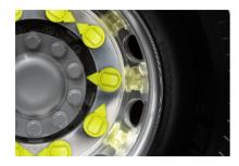
It's actually a clear-cut matter: The driver must make sure that the wheels and tires are in safe condition before setting off - this is what is written in the accident prevention regulations "Vehicles". In a commercial vehicle with several axles, this means an enormous amount of time and effort. With our innovation for the wheel nut indicator we provide a remedy.
