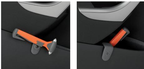
With this system you can mount the safety hammer on the inside of your car door. Rotate the small click-adapter for optimal positioning. It is possible to use the QUICK CLICK SYSTEM in combination with the PRO ADAPTER.
