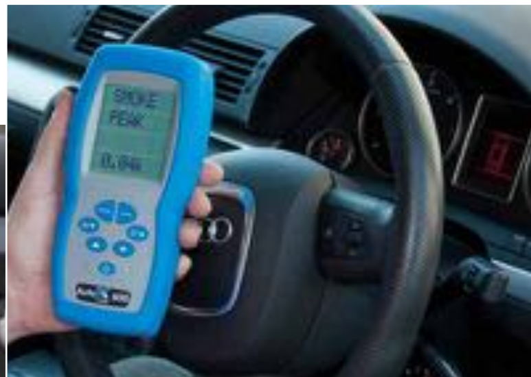
Car & commercial vehicle diesel engine exhaust smoke measurement
