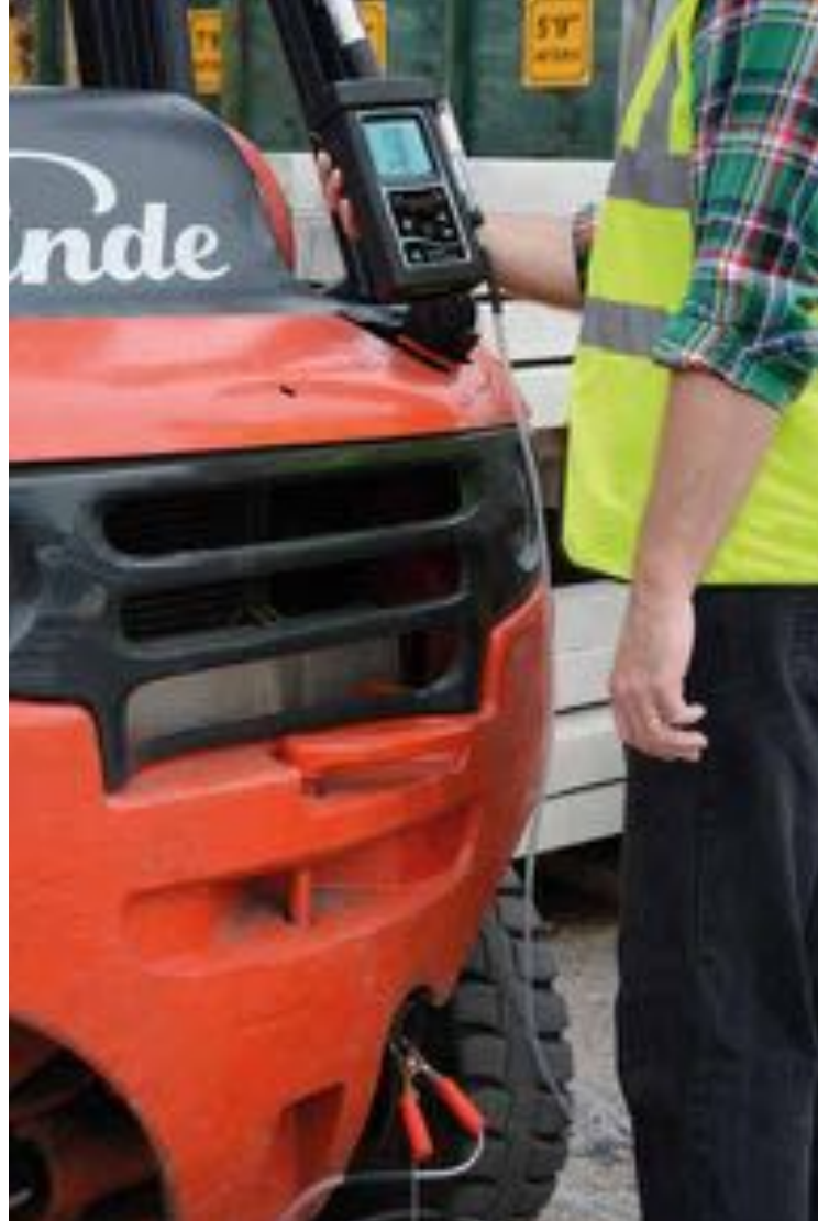
Fork lift truck exhaust emissions measurement
