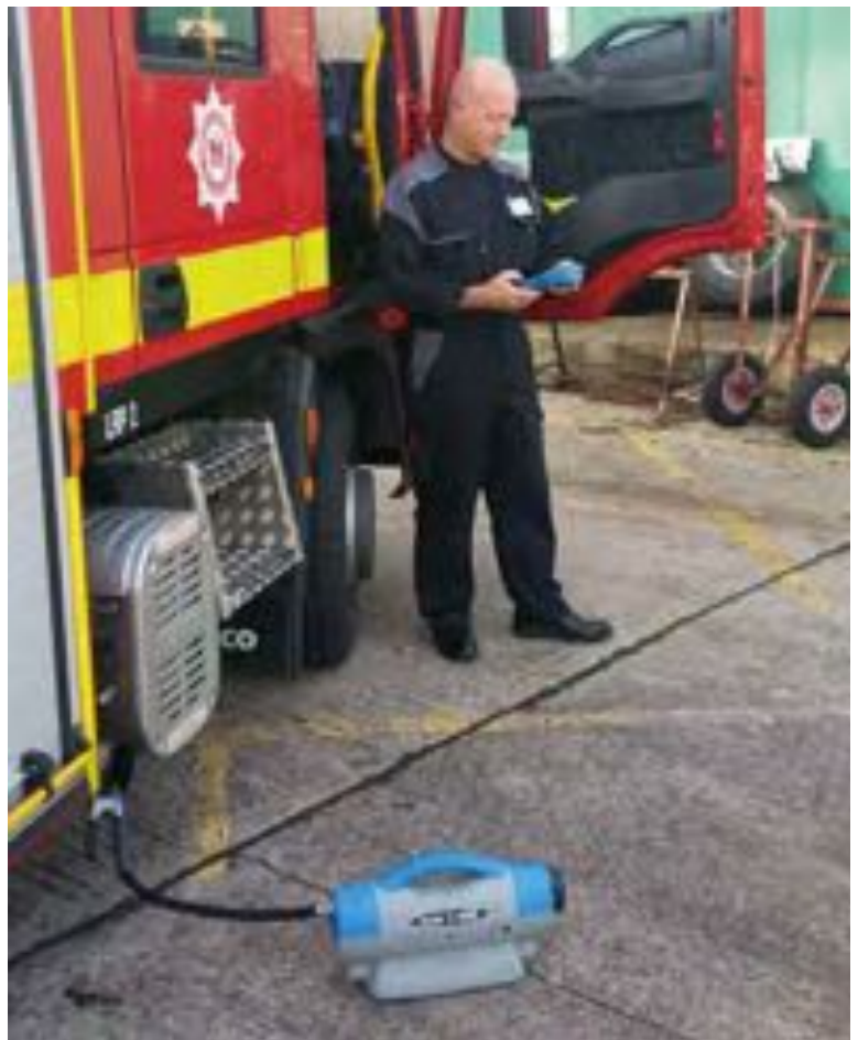
Wireless handset enables remote operation
