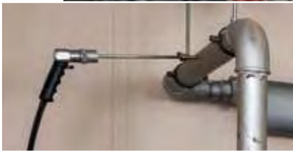
Gas Engine Testing with optional CHSP5 probe
