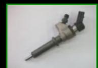
Injector Siemens Piezo
