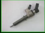
Injector Siemens Piezo
