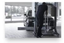
Adjust the upper reference panel to the height in accordance with manufacturer specifications (1.85 m for transporter). Exact positioning is made easier with the help of the spring relief.
