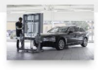
The calibration rig is mounted on a trolley. This makes it easy to move and adjust.
