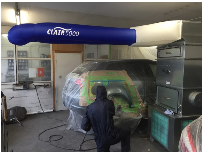
Extraction of paint mist on a painting table
