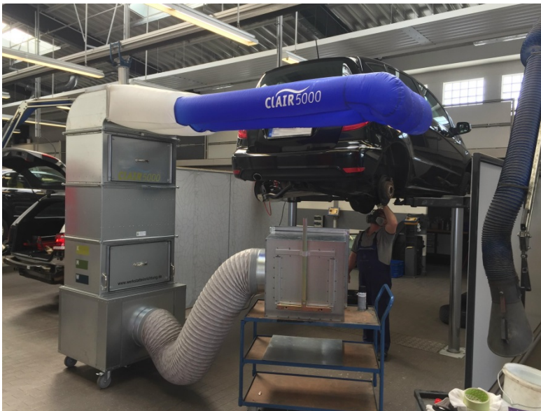
with hopper placed on trolley, e.g. for spraying underbody protection
