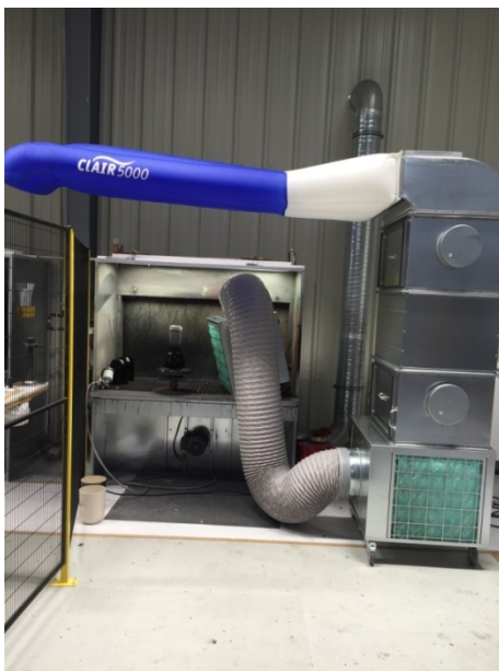
Extraction of paint mist on a painting table
