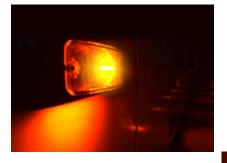
Using our control box the downlights can work together with the side-markers. They can flash with the direction indicators, and automatically come on and off according to the speed of the vehicle.
