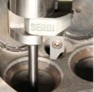
Built-in motorspindle paired with a 1.5 kW Siemens Inverter, with a maximum torque from 100 to 670 rpm and a maximum speed of 1200 rpm. Stator cooled by heat sink. Rigid heavy duty motorspindle of 80 mm (3.15") diameter for machining without chatter. Ensure a considerable machining accuracy thanks to a high precision tooth rack and a whole spindle assembly rigid and concentric to the valve guide.
