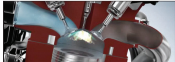
The GDI Combustion Chamber
