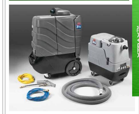
Huge 9 gal. solution tank with 1500 watt heater and 11.5 gal. recovery tank. Dual, twostage vacuums create 150" of water lift and 100 psi of 190°F cleaning solution. Swiveling lid allows easier accessibility within vehicle.
