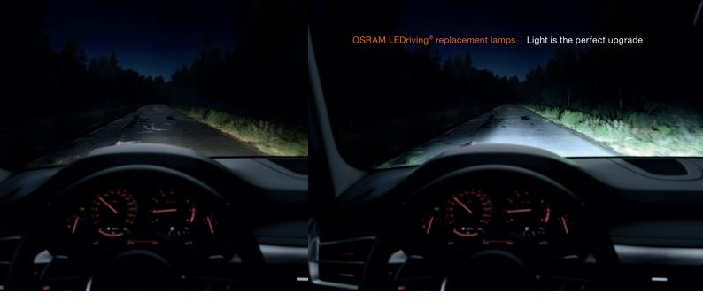
Daylight in the night: With a daylight-like color temperature of 6,000 K, OSRAM LEDriving® HL and FL lamps (right) provide a higher contrast and thus improve visibility.
