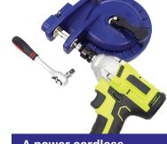
A power cordless /Pneumatic ratchet wrench can replace the included ratchet wrench to save time
