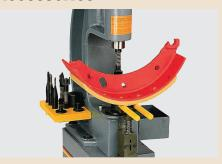
The brake shoe support holds the shoe in the correct position for riveting and deriveting, preventing it tipping.
