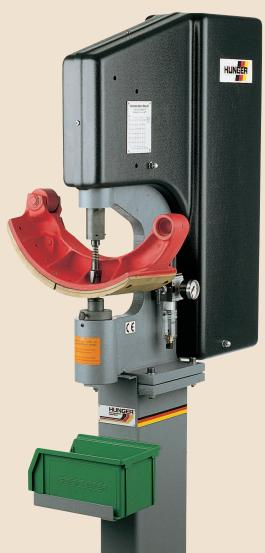
Accurate riveting of brake linings is an essential requirement for the safe operation of vehicle brakes and avoidance of a major source of brake squeal.
