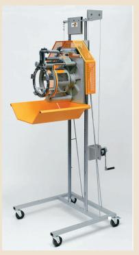
Machine with high trolley, working height 600-1600 mm for working on vehicles on a column lift.
