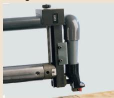
The tool slide is equipped with a digital read out which enables a faster, easier and faultless adjustment of the tools.
