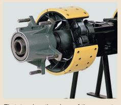
First, two locating rings of the correct size and the adaptor hub are fitted to the axle. Then the F 308 is attached to the studs of the adaptor hub. We can also supply suitable accessories for stub axles with mounted inner taper roller bearings.
