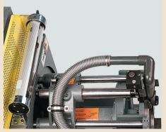
The optional machine lamp lights up the dark working area under the fender to make the mounting and adjustment of the machine to the axle easier.
