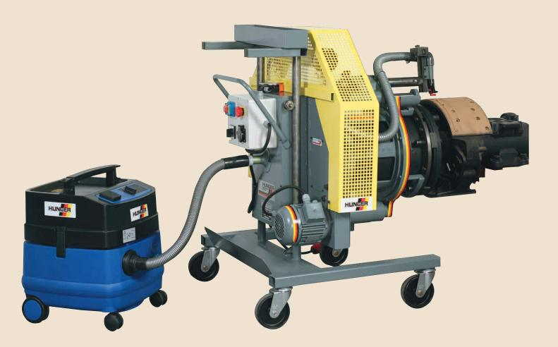
The profiling of brake linings in position, i.e. on the axle, guarantees safe braking values from the outset. Furthermore, the linings make contact over their full working surface. Overloading and consequent overheating caused by partial contact is eliminated and both brake lining and brake drum life extended.
