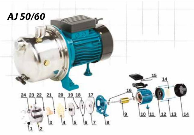
Single-stage self-priming centrifugal surface pump equipped with the Venturi tube  $\,$ system for increased suction capacity, designed for pumping of clean cold water from own intakes and for increasing pressure. Sections of pump body and shaft that come in contact with water are made of stainless steel (INOX design). The pump has a power cable with a plug. The pump motor is provided with thermal protection.
