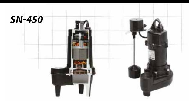
Submersible pumps designed for pumping sewage, dirty water, and water from flooded premises. SN-450 pump is made of cast iron with VORTEX-type impeller. It can pump water with mechanical impurities with particle diameter of up to 20 mm. The pump is equipped with a vertical float switch for easy automatic operation in 25 cm diameter wells. SN-450 pump is equipped with thermal protection mounted in the motor winding.
