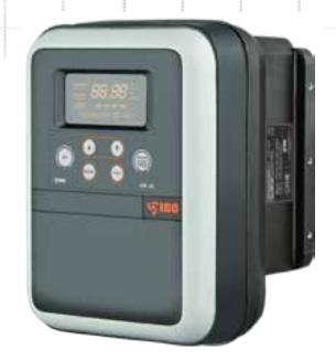
Thanks to real-time pressure analysis, the inverter adjusts the rotational speed of a pump to system's demand at a given time. Variable rotational speed of the pump stabilises pressure, thus reducing water and current consumption.
