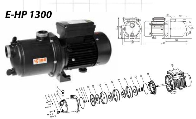
The pump used for clean, cold water from own intakes and for pressure boosting. The HP pumps are multistage, self-sucking surface pumps with increased suction capacity provided by a Venturi tube. The pump shaft is made of stainless steel (INOX). The pump is top quality in terms of workmanship and materials. It features a power cable with a plug, and the motor has integrated thermal protection.
