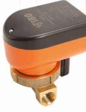
Seal-less circulation pumps designed for forcing hot water circulation. In systems without hot water pumps, after opening the tap, before the hot water starts flowing, cool water remaining in the pipeline will flow first. If a hot water pump is installed, hot water will flow almost immediately after opening the tap. The pump is usually installed upstream the boiler or hot water tank. With years of experience, we have been able to improve previous designs and create the top quality pump.
