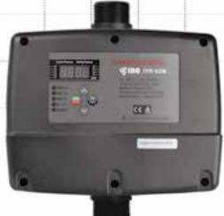
IVR-02M Intelligent Pump Controller is an easy-to-use control and protection device for direct connection of 0.75 KW to 1.5 KW (from 1 HP to 2 HP) single-phase submersible pumps, surface pumps, deep well pumps, etc., maintaining a constant, set water pressure by changing the rotational speed of the pump motor.
