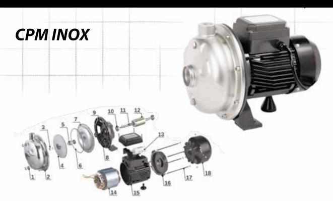
Single-stage non-self-priming centrifugal pumps designed for pumping non-aggressive liquids with non-abrasive and non-absorbent solids content of 0.27 kg/m $^3$ . The maximum temperature of the pumped liquid is up to 60°C. The pump motor is provided with thermal protection mounted in the motor winding. Hydraulic parts that come in contact with water are made entirely of stainless steel.
