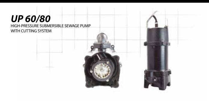
The UP60/80 pumps are equipped with a two-stage hydraulics to increase the maximum pressure. An important feature of KRAKEN 1800 is a multi-channel disk cutting system designed to minimize the risk of clogging. In addition, the outlet is threaded in order to connect a pipeline or fast connection. The pump is supplied with thermal protection mounted in the motor winding.
