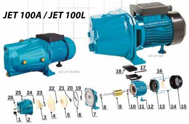
Single-stage self-priming centrifugal surface pump equipped with the Venturi tube system for increased suction capacity, designed for pumping of clean cold water from own intakes and for increasing pressure. The pump body is made of durable cast iron, and the pump motor is provided with thermal protection. The pump has a power cable with a plug. The pump is available with accessories or in the booster set.
