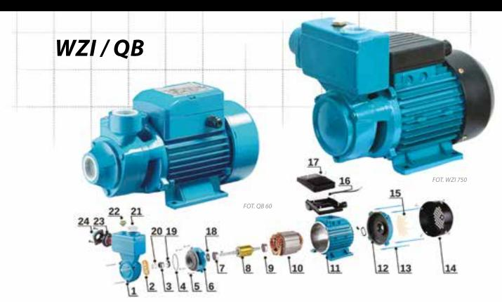
Single-stage self-priming peripheral surface pumps for pumping of clean cold water from own intakes and for increasing pressure. Pump impellers are made of brass. The pump body is made of durable cast iron with the built-in non-return valve. The pump motor is provided with thermal protection. The pumps have a power cable with a plug.
