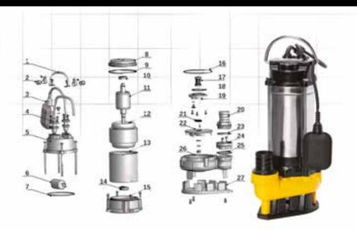
Submersible pumps designed for pumping sewage, dirty water, and water from flooded premises. The pumps are equipped with float switches for automatic pump control. Threaded outlet connection and a set of adapters provide connection of the discharge hose with a hose clamp or fast-connection coupling. WQF pumps are equipped with thermal protection mounted in the motor winding. The motor housing is made of AISI304 stainless steel, and the impeller is made of grey cast iron.
