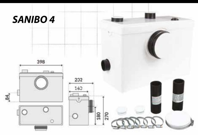
SANIBO 4 is a high quality fully automatic toilet pump for pumping sewage, equipped with three inlets for draining sewage from toilets and wash basins/sinks - one main 100 mm inlet for toilets, 40mm for shower bases or wash basins, and one 40mm outlet. It has a switch for automatic pump control - the pump automatically stops after filling the device. Additionally, the pump can be started manually.
