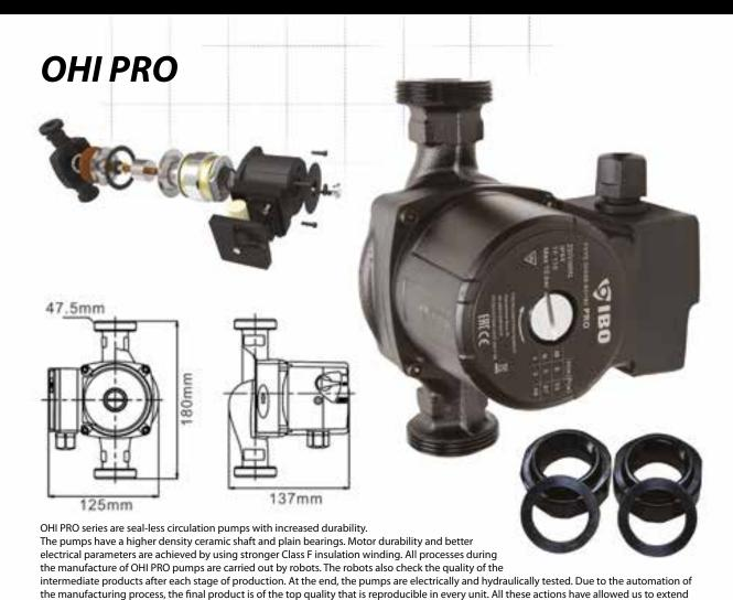
By default, the pumps have 3 speed levels for adjusting operating parameters depending on the user's and system's requirements. Due to the design and high quality materials used, the pumps are very quiet during operation.
