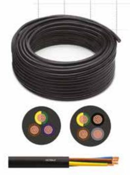
H07RN-F rubber heavy duty power and control cable 450/750 V, for in industrial and agricultural applications. Class 5, from -25°C to  $60^{\circ}$ C, oil resistant, flame retardant
