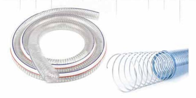
Transparent light weight steel-wire-reinforced small-bend-radius hose. Reinforced hoses are used as suction and discharge hoses. They are resistant to negative pressure and can be used in adverse weather conditions.
