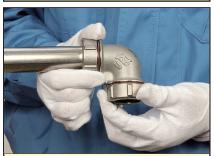
**8**.Set the conical washer to a section where the cap nut side surface comes in contact with the fitting and tighten the nut until the colored surface is not visible.
