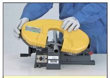
**l**.Referring to the pipe cutting dimension table, cut the pipe at a right angle to the axis core with a metal saw or band saw.
