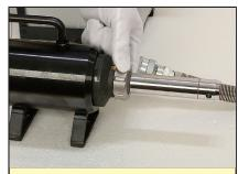
**3**. Tighten the cap nut to the yoke.
