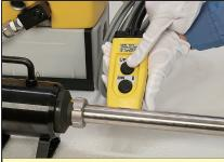
**5**.For the pipe expansion work, keep pressing "UP" button until the motor stops.
