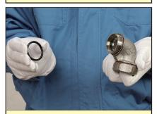
**7**.In case rubber sealing material is dropped, be sure to mount it to the fitting main body.
