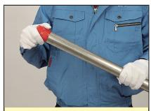
2.Carefully, remove burrs from both the inner and outer chamfered surfaces carefully using reamer, sand paper and grinder.
