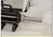
**4**.Insert the pipe into the guide rod completely.
