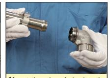
**6.**Insert the enlarged pipe into the fitting and tighten the cap nut.
