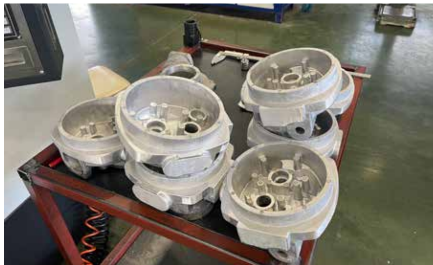
— 150 nM electrical actuator parts before machinery
