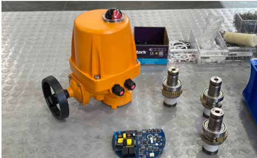
— 60 nM electrical actuator and gears and electronical cards
