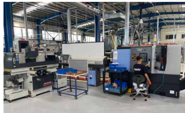
— Solenoid valve core manufacturing cell
