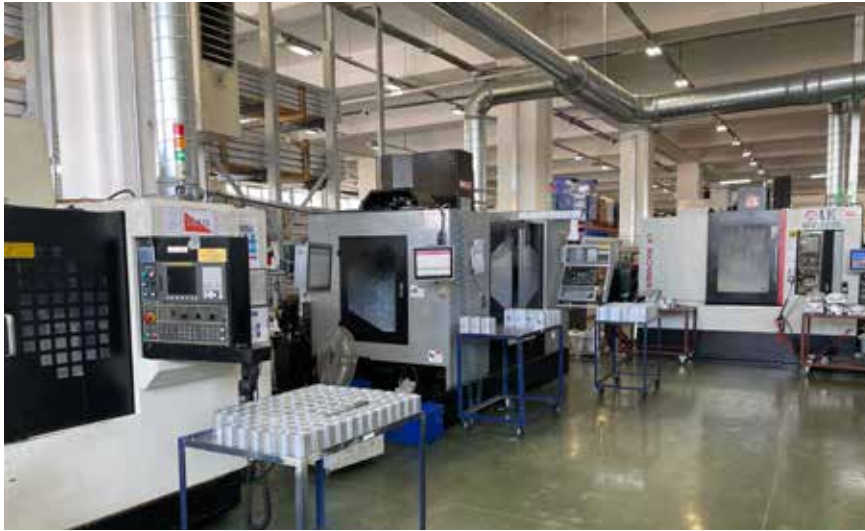
— Vertical cnc center cell for electrical and pneumatic actuator body manufacturing
