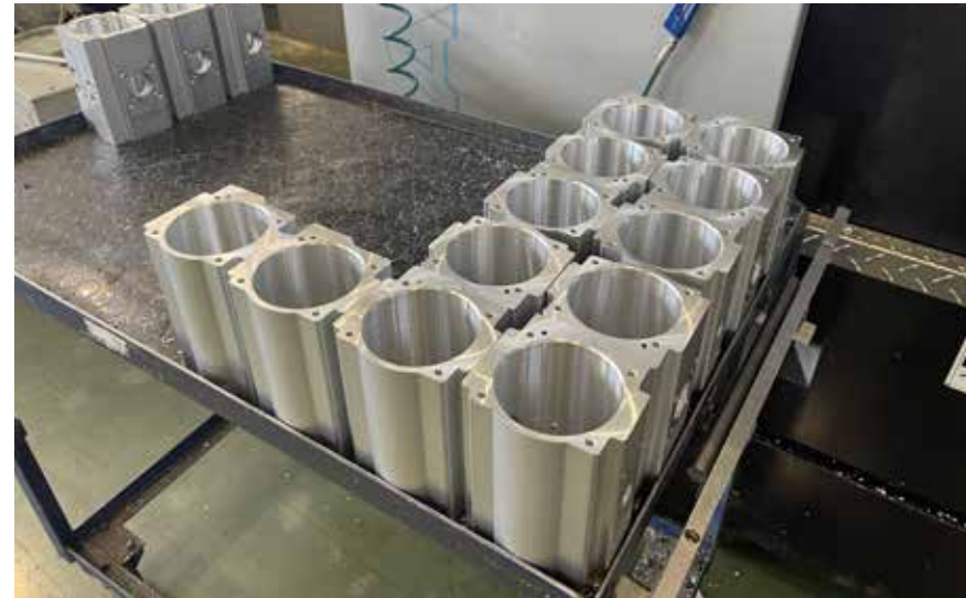
— Pneumatic actuator body after machinery
