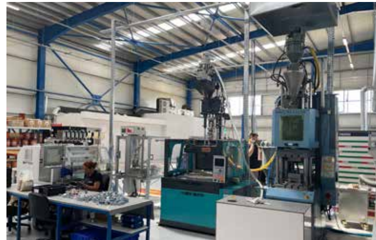
— Coil winding and plastic injection cell
