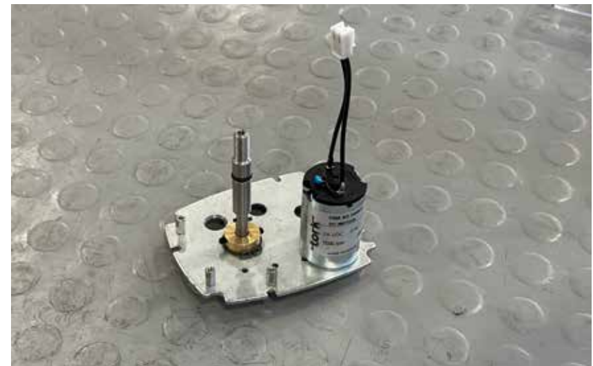
— 40 nM electrical actuator motor and shaft before assembly
