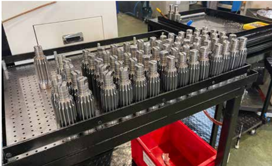
— Pneumatic actuator pinions after machinery
