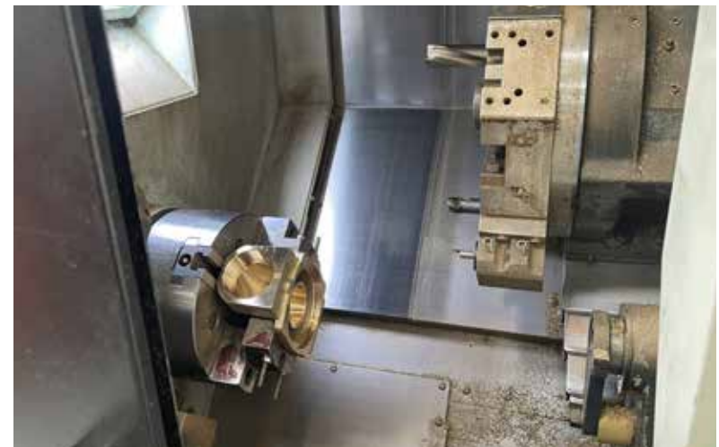
— Solenoid valve cnc machining
