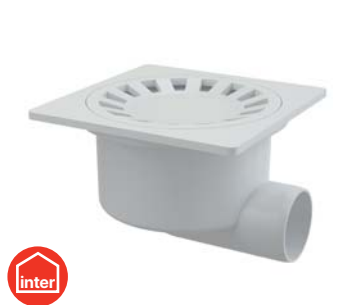
APV15 Floor drain 150×150/50 mm side outlet, white grid, wet odour trap
