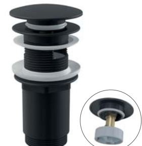
A392BLACK Wash-basin CLICK/CLACK waste 5/4", metal with overflow, big plug black-matt
