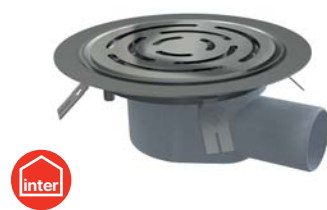
APV3513 Floor drain 105×105/50 mm side outlet, stainless steel grid, stainless steel flange and collar-2nd level insulation, combined odour trap SMART
