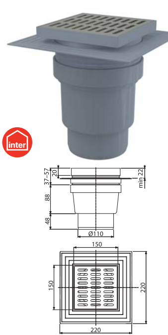
APV13 Floor drain 150×150/110 mm straight outlet, stainless steel grid, collar-2nd level insulation, wet odour trap
