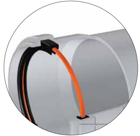
Collar interval in the installation of PVC Duplex Pipes and Fittings should be 1 m.
