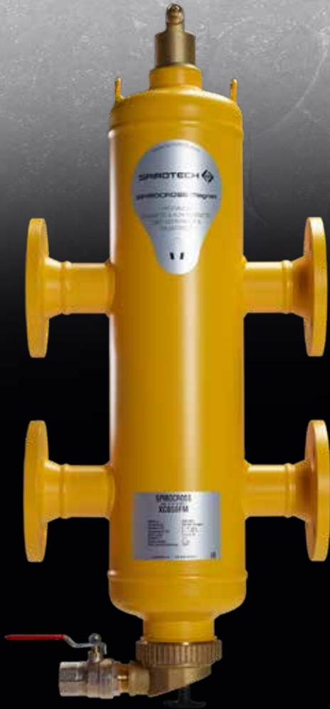
In chilled water systems it is often necessary to hydraulically decouple the primary circuit (cooling supply) from the secondary circuit (cooling consumer). This means that the two circuits do not influence each other. This feature is necessary to maintain a constant volume flow via the chillers, whereas the volume flow via the consumers is variable due to changing load.
