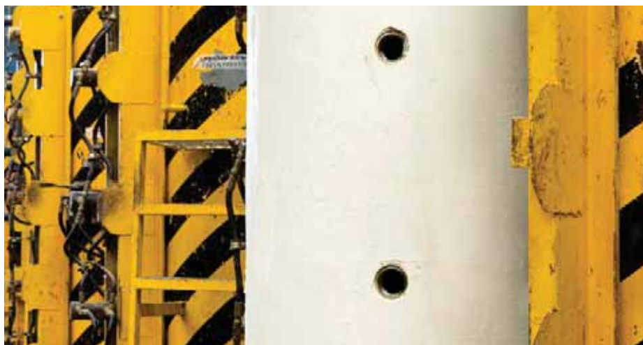
Rigid, mould-injected PU insulating material
