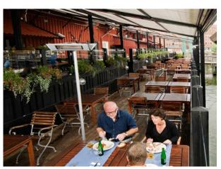
Post for floor mounting available as an option. With a triple bracket, three infrared heaters can be positioned on the same post so that heat can be directed in all directions.
