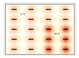
Plan sketch: Temperature zones with radiant heaters.
