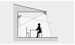
The heaters should heat from at least two directions for an even heating.
