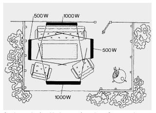
Good example of positioning, seen from above. Output requirements approx.  $1000\,\text{W/m}^2$ .
