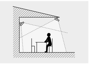
The heaters should heat from at least two directions for even heating.
