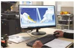
Using CAM software we can simulate, optimize, plan and verify the correct machining of the products on the different machines. To implement that successfully it is necessary to have a great experience and knowledge.
