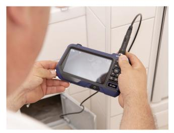
Large 5" screen Moisture under the bathtub? With the Wöhler VE 400 the cause is quickly found.
