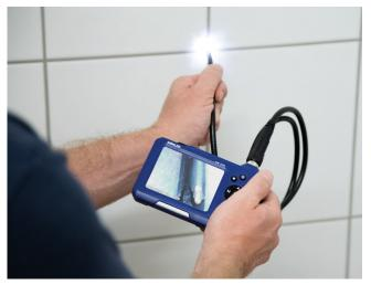
View through smallest openings Just a  $\varnothing$  6 mm opening in a tile cross is sufficient to view the installation behind the wall (in the picture Wöhler VE 320).
