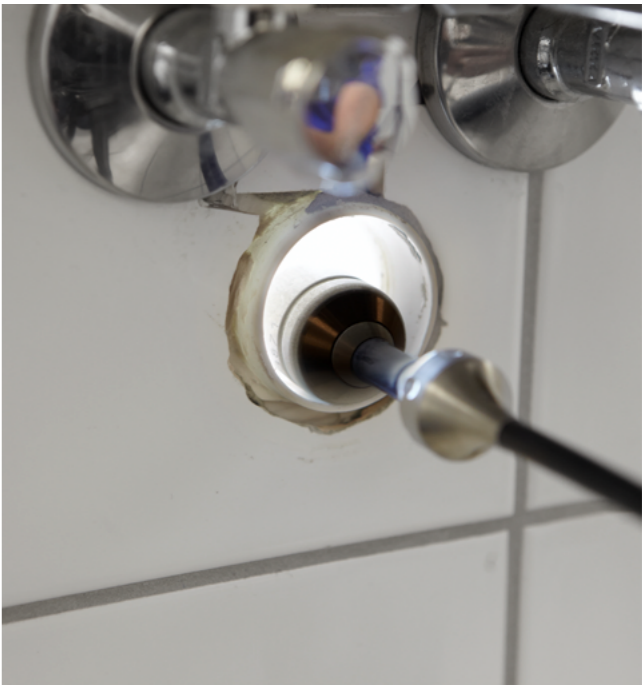
The robust color camera head is waterproof to IP 68 rating. With a diameter of just 26 mm it easily negotiates bends in ducts of Ø 40 mm and larger.
