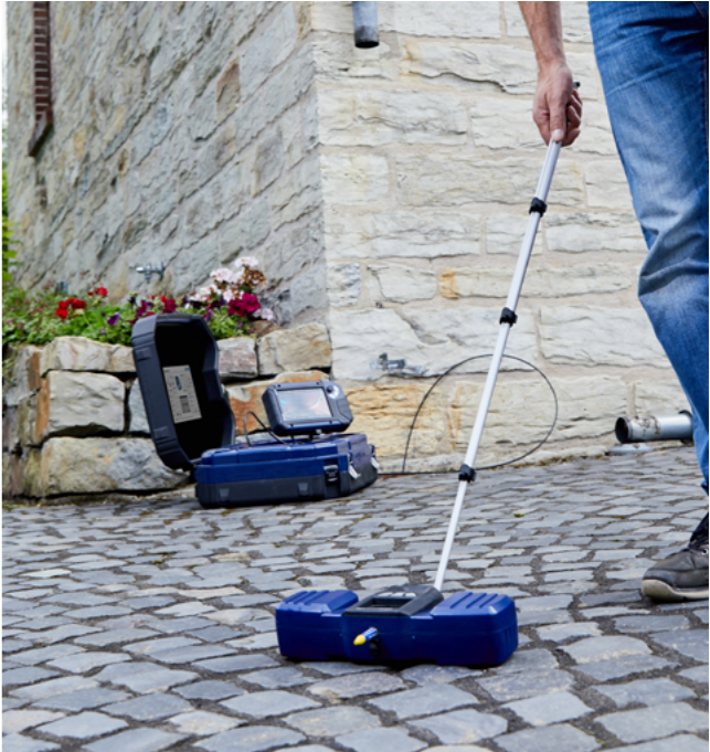
Precise location of the camera head with the Wöhler L 200 Locator.
