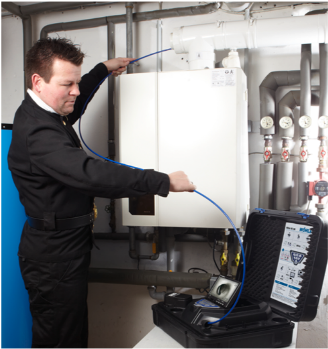
The 360° pan and 180° tiltable color camera head easily negotiates 87° bends.
