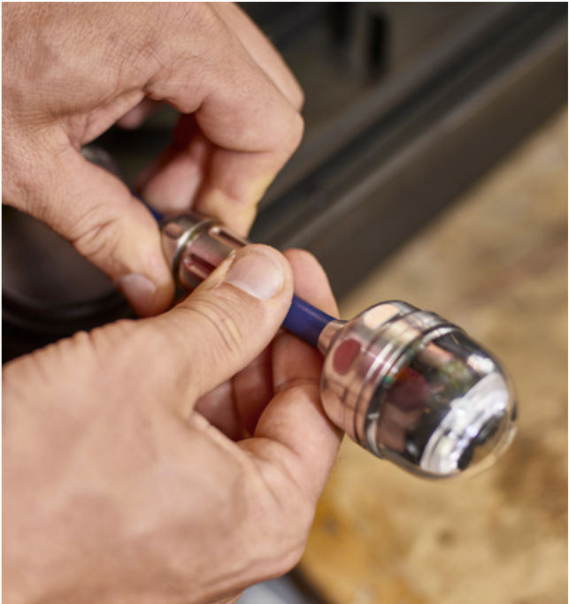
Thanks to the excellent lighting system of the detachable, color camera head, the camera supplies razor sharp images of even the darkest corners of the section under inspection.
