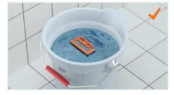
Well thought out: The Fuginator® can be sterilized and is acid- and lye-proof. It floats, so as to be easily retrieved from a cleaning bucket.
