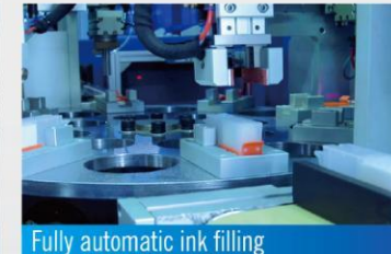
Fully automatic ink filling
