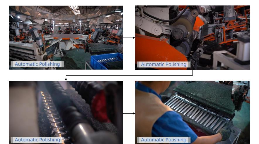
Multi-stage rotary automated polishing machines
