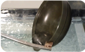
The product is intact after the thermal shock test
