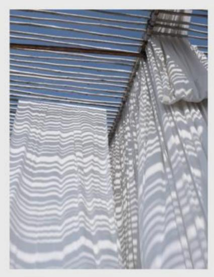
The above tall structure made of bamboo allows yards of washed and/or dyed fabric to be hung in broad daylight for drying before being rolled into a "thaan" for further printing processes.
