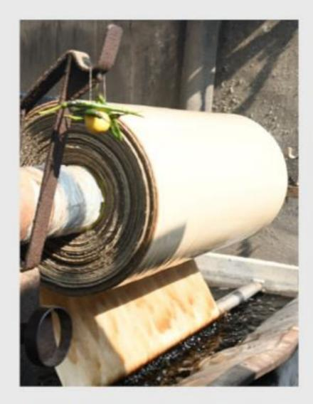
Rotary dyeing allows yards of grey fabric to be dyed uniformly in desired colours before they proceed for printing. This process is sustainably articulated for the water and dye to be circulated through the fabric and squeezed out by centrifugal force.
