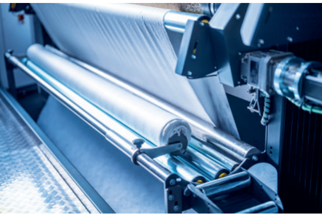
▲ Quick change system for ticking
