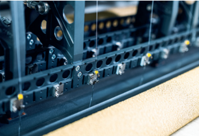
▲ Quick change sytsem needle and loopers
