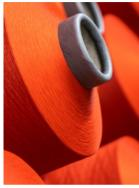
By incorporating colour during the extrusion and spinning process, we obtain solution dyed yarns and fibres with excellent regularity and colour fastness. This process achieves significant savings in terms of water and energy consumption when compared to dyeing in an aqueous medium.
