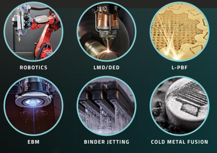
In addition to powder bed processes, technologies include axis-controlled and robot-controlled deposition welding (LMD/DED) as well as other processes such as EBM, Binder Jetting and Cold Metal Fusion.
