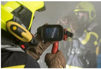
Thermal imaging cameras (TIC's) for firefighters produce an image of the intensity of the thermal radiation detected. Each colorization mode has its own color palette.
