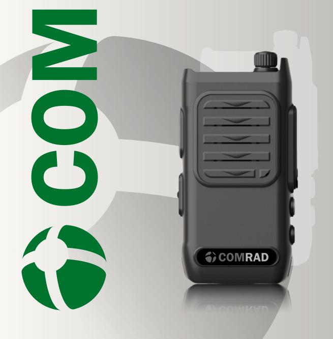
The multifunctional portable Android terminal Comrad CP10 is a subscriber device of the intercom system in a group or between subscribers. In particular, it can be used in a PoC (Push-to-Talk Over Cellular) system using cellular network and/or WiFi network to organize communication with protocol subscribers using PTT (Push-to-Talk) technology.
