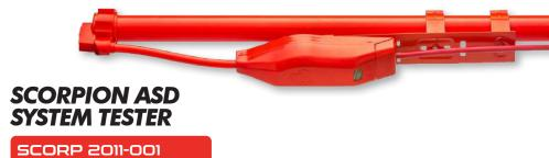
The Scorpion head unit is permanently mounted adjacent to a sampling point on an ASD system pipe - typically at the end of the run. Just one head unit is required for each pipe run regardless of the number of sampling points.
