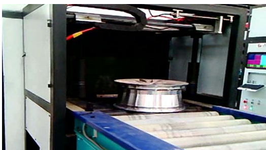
Automatic Dynamic balancing online testing
