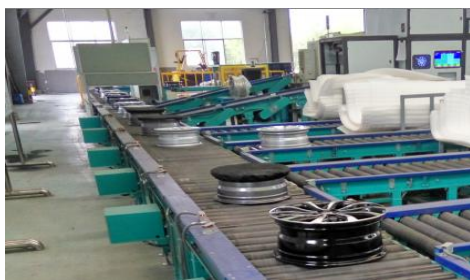
Adopting image recognition system in packing line.
